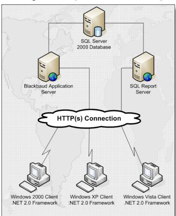
After you understand the basic setup, you can plan larger-scale and more advanced deployments. The Infinity platform is scalable, and can accommodate large organizations with complex networking needs. For example, failover servers, load balanced web servers, and firewalls can be used for more robust and secure installations.
